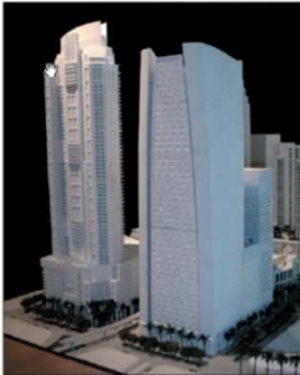
The Realization Group used the ZPrinter 310 Plus to create this 28-inch-high model of "The Met" in Miami, in one-fourth of the time and cost of traditional architectural modeling methods.
